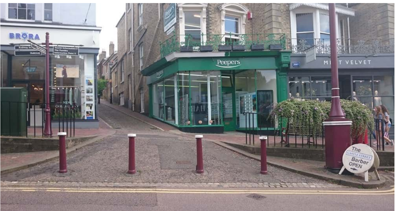
Figure 28: Example of existing modally filtered street in Tunbridge Wells. Photo: Bartholomew Wren.
