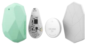
Figure 4: Exploded diagram of an Estimote beacon, showing its small interior board and CR 2450 battery
