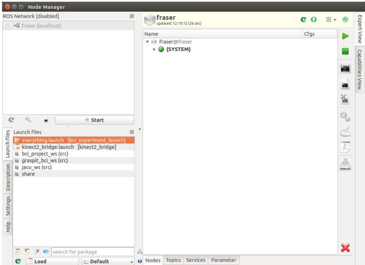
To start the controller - in the *Launch files* tab on the bottom left of the window, navigate to the file 'bci\_project\_ws/bci\_experiment\_launch/everything.launch' and double click. Click 'OK' in the popup window. Highlight all the nodes by shift-clicking the first and last node and click the green play button in the top right:
